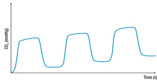
**Figure 8.** Capnogram demonstrating re-breathing of CO<sub>2</sub>; note the baseline does not return to zero. In such cases, the anesthetic circuit or ventilator should be checked, as this is a technical problem.
